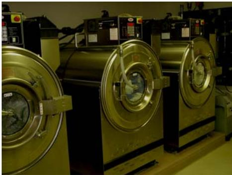
*OZONE* carries an electrical/chemical charge in the washing solution, which actually starts to dissolve soil on contact. This process activates the chemicals in cold water instead of using hot water at 140-160 degrees.
